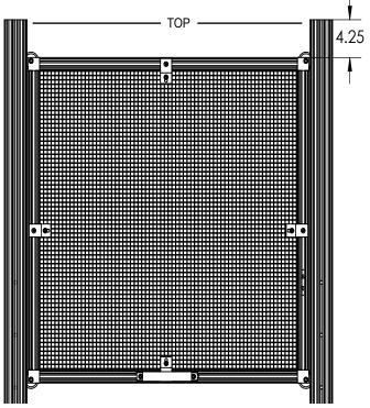
Place the screen assembly between the frames that were laid out in step 14. Make sure that the screen assembly is approximently 4.25 inches from the top of the frame.
