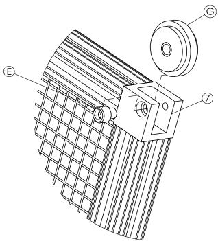
Place part G in 7 so that the hole in G lines up with hole of 7, bolt in place with E.
