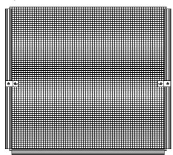
Put screen into middle slot on one of the sides of one part #4.
