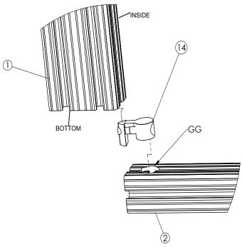
Slide part # 14 into inside bottom of part #1 (Part #14 may need to loosen bolt). Slide part #2 in between part #1 and other outer frame piece, allowing for circular part of 14 to enter hole GG. The bottom of part #2 should be level with the bottom of part #1.
