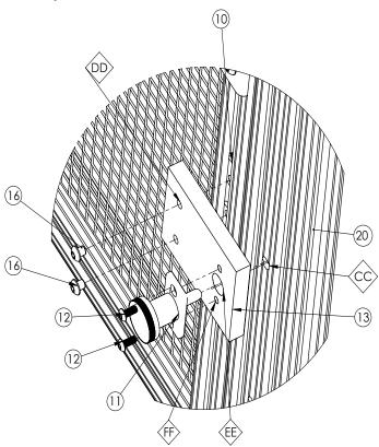
On right hand side of screen frame line up hole DD with holes of the 2 part #10's. Line up hole EE with hole CC on outer frame, using part #16 bolt part #13 to screen assembly. Put part #11 in hole EE bolt with part #12 to part #13.
