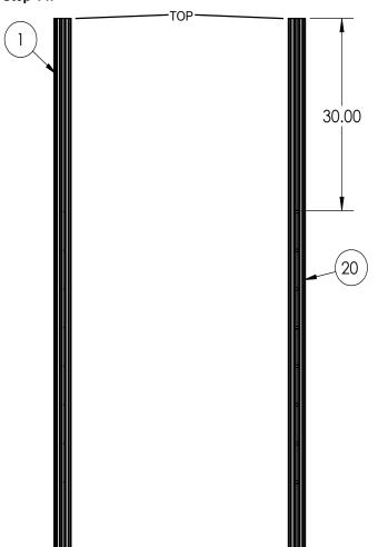
Lay out part #1 and second outer frame piece with holes; lay the frame piece with the holes 30 inches from the top.
