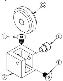
Disassemble part #7, unbolt part E from part #7 then remove wheel (G) to access the two bolts (F), remove F.
