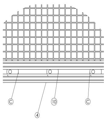
Slide in one part C (that comes with handle) in part #4 (same as in step 2). Slide in a part #10 to the middle of #4. Attach part #9 using step 3. Then slide in the other part C after part #10.
