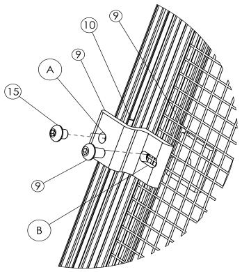
Line up hole A with hole in part #10, make sure hole B is not over the hatching of the screen. Bolt part #15 into hole A and part #10. Use bolt that comes with part #9 slide into hole B and bolt the black plate of part #9 (on the back side of the screen).
