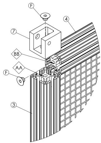
Line up holes that the F bolts came out of with hole AA on a part #3 and hole BB on a part #4. Using bolt F (that comes with part #7) bolt part #7 on frame.
