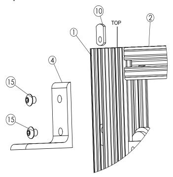
Slide two part #10's in the top of the outer most slot on part #1, make sure that the extruded part of #10 is facing the front of the frame assembly as it slides in. Line up part #4 (on the outer slot of part #1) with the bottom of part #2. Use two part #15 to bolt part #4 to part #1. Do this for both sides.
