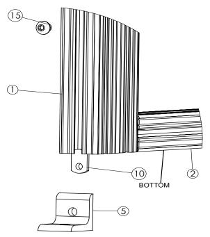
Slide 1 part #10 into the outer part (1.5" side) of part #1 4.5 inches up. Line up the hole on part #5 and bolt on using part #15
