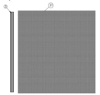
Put the screen in the middle slot on one of the sides of part #3.
