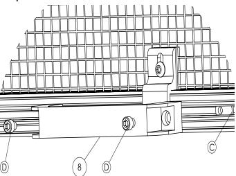
Move parts C so that part 8 is centered above part #9. Bolt part #8 to part #4 using bolts D that comes with #8.
